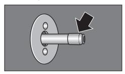
The part which connects the brew unit and the central spout is located on the inside of the machine door.
